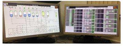
The system comprises nine silos, 30 day bins, 12 mixers and six blowers. Raw ingredients, including flour and sugar, are transferred from the silos to the day bins. They are then weighed into the mixers, using recipe and route control.
